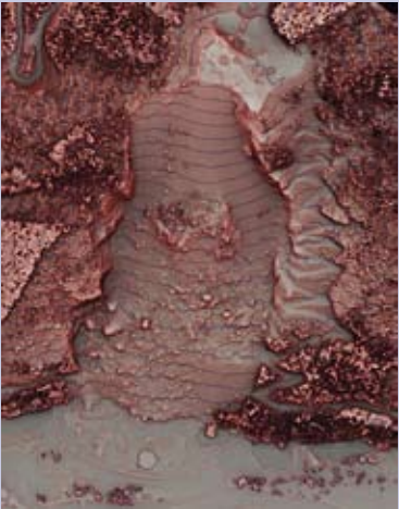
Takahashi-river 0.5m DSM data from LiDAR. Shape of boulders in the slope failure are displayed
