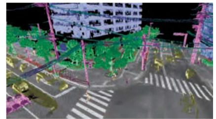
AI-Driven Automated Classification of Ground, Vegetation & Buildings
