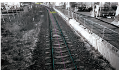
Point cloud laser scanning and automatic extraction of features using RailLis
